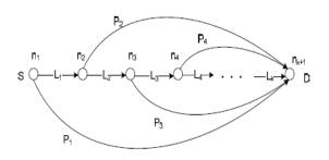
Figure: The major route consists of L1, L2,..., Lk. Each node in the primary route ni, has an alternate path Pi to the destination. Alternate routes in [18].
